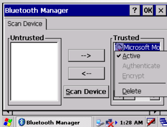
Figure 13 Moving a device to the Trusted box
