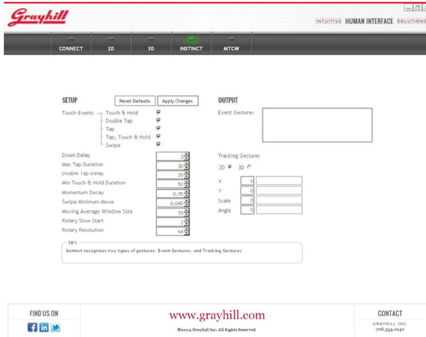
The Instinct Page demonstrates the Instinct Gesture Recognition process by allowing the user to change some of the settings that control how gestures are recognized - and then allowing the user to observe how these changes affect the output. After changing one of the settings, hit the “Apply Changes” button to try out the new settings. Default settings can easily be recovered by hitting the “Reset Defaults” button. The current settings are retained for use with any of the other demo screens.
