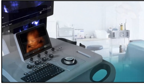
On this ultrasound panel, a Touch Encoder replaced four switches, a trackball and eight buttons.
